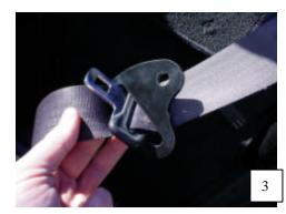
4. Unbolt the stock seatbelt guide from the rollbar tab using a 9/16" wrench.
