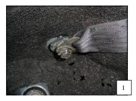
2. Position the hole toward the rear of the car, with the fat end toward the inside of the car (driver's side shown). Insert the anchor end of the seatbelt upward through the slot in the seatbelt adapter (see photo).
